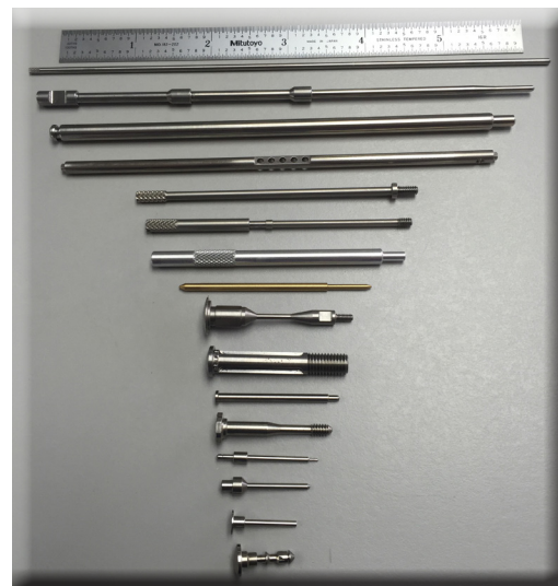
Long parts produced on the Citizen Machines at Pacific Swiss
